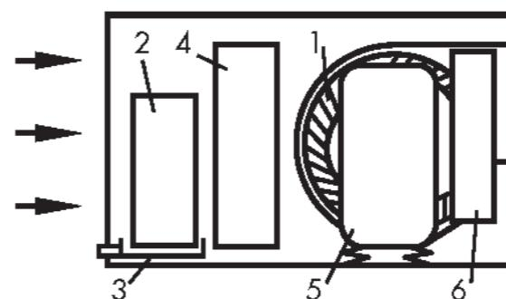
The fan (1) sucks the humid air through the evaporator. There the air is cooled and the moisture in the air condenses into water. This water is collected in the tray and drained away through the sump and piping.
